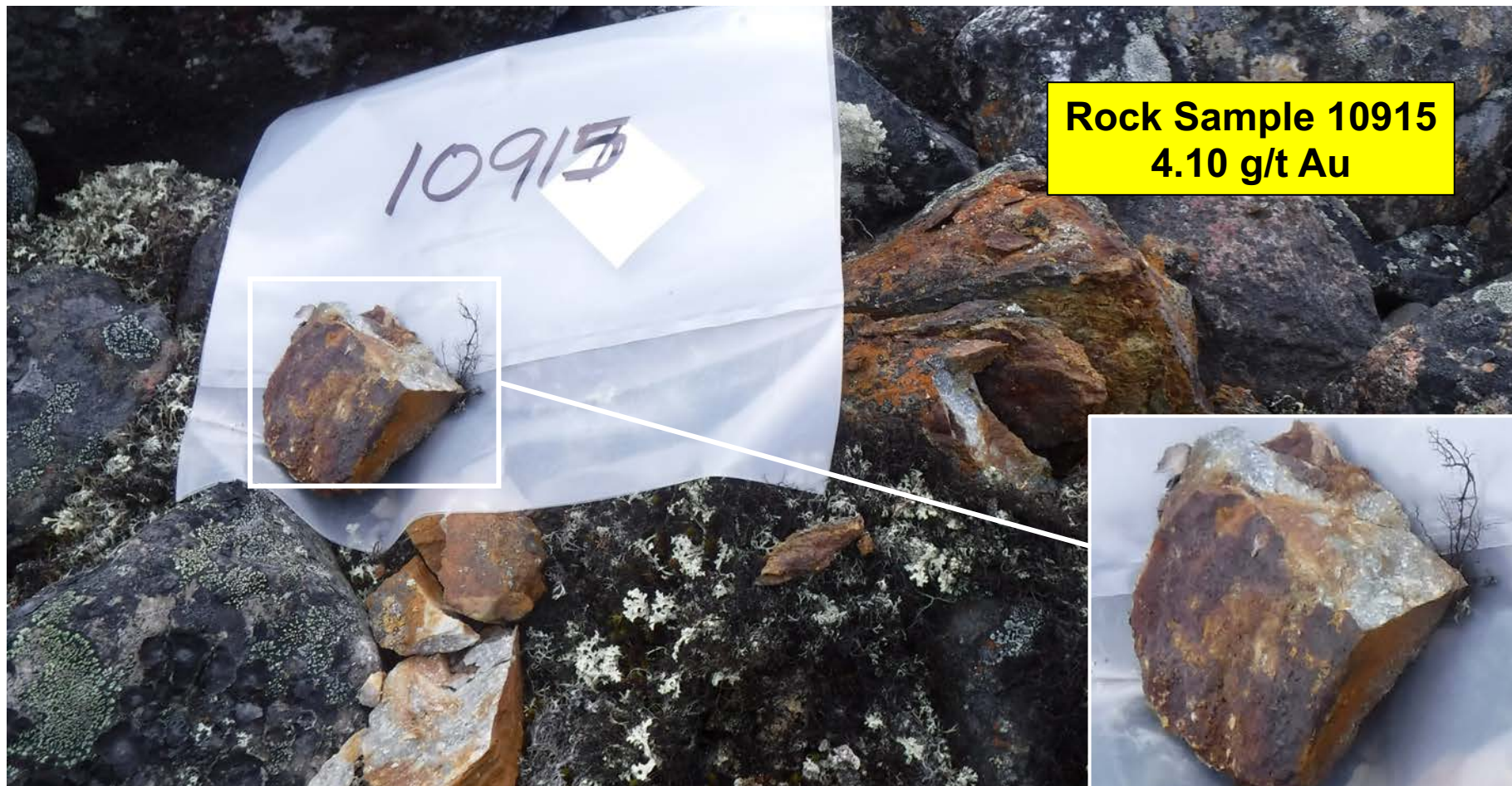
Oxidized boulder (felsic volcanic) - Gold hosted mineralization within strong silicification containing disseminated pyrite-arsenopyrite
