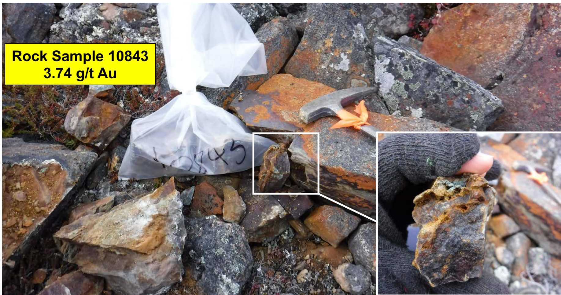
Shear-zone hosted gold mineralization - Highly oxidized boulder with quartz veins hosting pyrite-arsenopyrite
